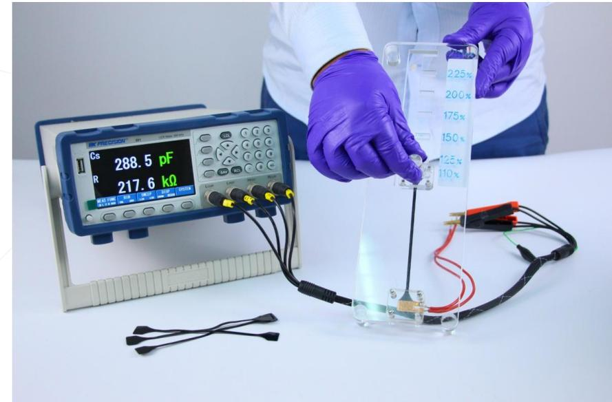
**Compo-SiL<sup>®</sup> - Capacitive stretch sensor**
